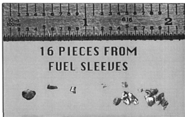
Fig. 7b Sixteen metallic fragments retrieved from fuel sleeves.
